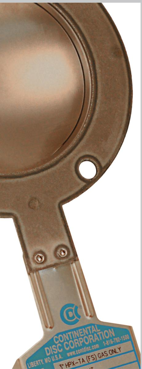
The HPX-Ta™ Rupture Disc is a Tantalum semicircular scored reverse acting rupture disc designed specifically for use in highly corrosive media, such as bromine, chlorine, HCL, nitric acid or sulfuric acid. In certain concentrations, temperatures and moisture conditions, Tantalum is frequently the only suitable rupture disc material for the application.
